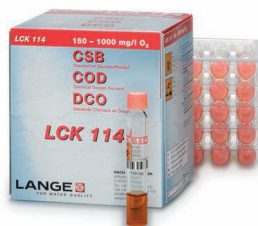
Cuvette test LCK 114 for the determination of COD
