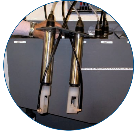
Fig. 4: pH and Redox sensors with automatic cleaning system
