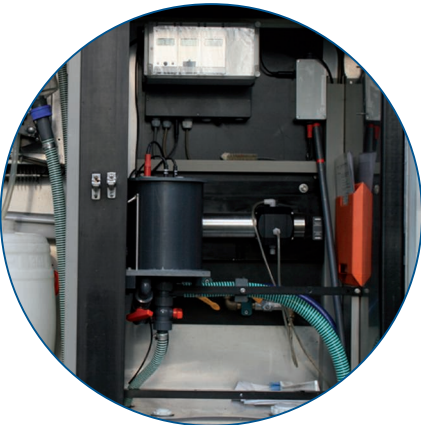
Fig. 1: NITRATAX plus sc nitrate probe (bypass), mounted in the sampler unit
